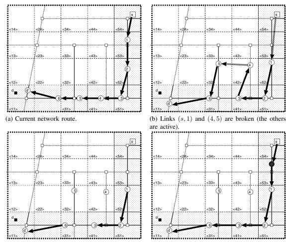
(c) Nodes outside the grid sequence and associated links are removed from network route.
